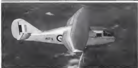
"ZIPPER WING" IN FLIGHT —New in flight plans of wood strib being tested by the Lockheed personnel on a modified DC-6B glider to explore boundary layer control. Continuous slot on top of wing seals off air. Slots near trailing edge appear to be ribs for test purposes.
